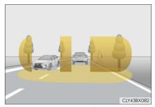
• Adjusts the distance that the low beams are projected according to the distance to a preceding vehicle.
