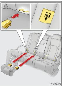
4 After installing the child restraint system, rock it back and forth to ensure that it is installed securely.  $(\rightarrow P. 68)$
