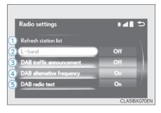
When traffic announcement is set to on, the tuner will automatically seek a station that regularly broadcasts traffic information and the station will broadcast when the traffic information program starts.
