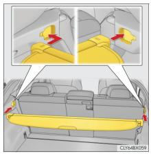
2 Pull out the luggage cover and hook it onto the anchors.
