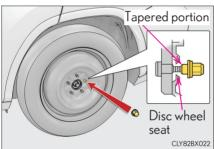
Tighten the wheel nuts until the tapered portion comes into loose contact with the disc wheel seat.
