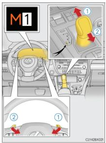
When in the M position, the gear will not change unless the shift lever or paddle shift switches (if equipped) are operated.
