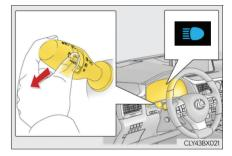
**2** Press the Automatic High Beam switch.
