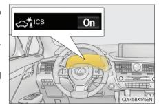
When the Intelligent Clearance Sonar is disabled, the ICS OFF indicator illuminates.
