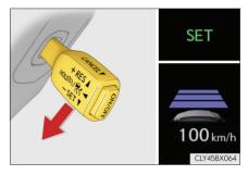
If the lever is operated while the vehicle speed is below approximately 50 km/h (30 mph) and a preceding vehicle is present, the set speed will be adjusted to approximately 50 km/h (30 mph).
