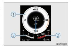
③ Engine oil pressure gauge Displays the engine oil pressure. A buzzer will sound and warning message will be displayed if the engine oil pressure becomes low. (→P. 675)
