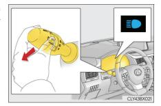
**2** Press the Adaptive High-beam System switch.
