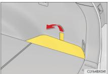
Pull the strap upwards when lifting the cover up.
