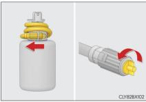
3 Connect the hose to the valve. Screw the end of hose clockwise as far as possible.
