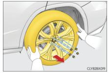
Vehicles with a full-size spare tire: Remove the wheel ornament by pushing from the reverse side.
