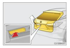
A buzzer will sound and the power back door will automatically open.
